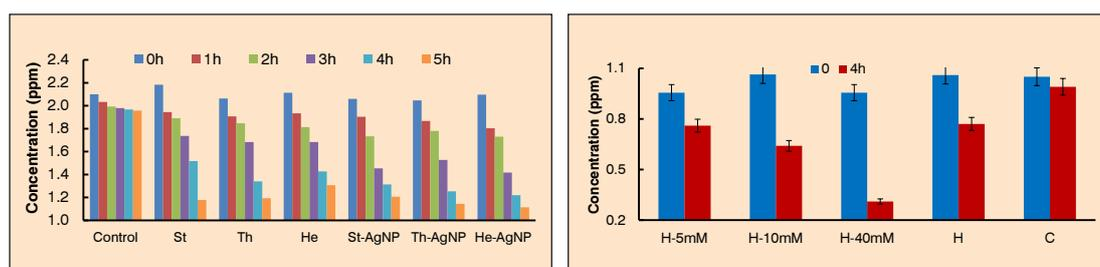
Fig. 2.26. Ammonia removal activity of native zeolites and heulandite and silver ion exchanged heulandite with and without silver nanoparticles
