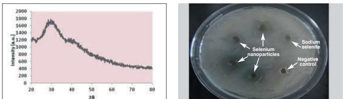
**Fig. 2.30.** XRD pattern of biologically prepared selenium nanoparticles antibacterial activity of selenium nanoparticles against *Aeromonas hydrophila* synthesized
