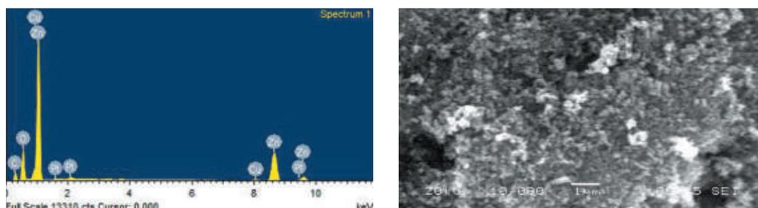
Fig. 2.27. SEM photograph of prepared zinc oxide nanoparticles
