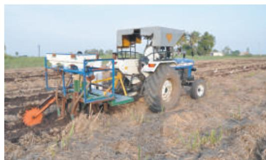
**Fig. 5.3.** Stubble shaving, Off-barring, Root pruning and Placement of basal dose of fertilisers
