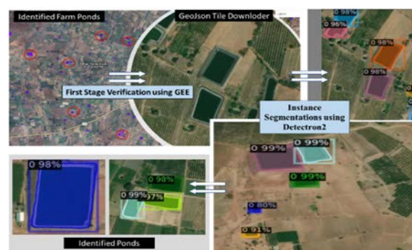
Fig. 2.1.15: Methodology for identification of farm ponds and storage water tanks using satellite imagery and deep learning
