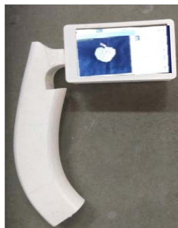
Fig. 2.3.28: Prototype Device for detecting custard apple maturity
