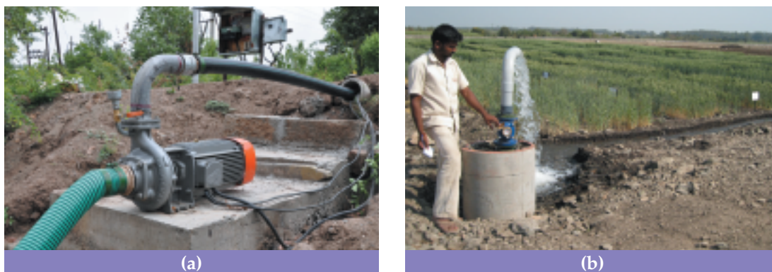
Fig. 2.7. Remotely controlled irrigation pump located 2 km away from NIASM (a), monitoring irrigation with water meter (b)
