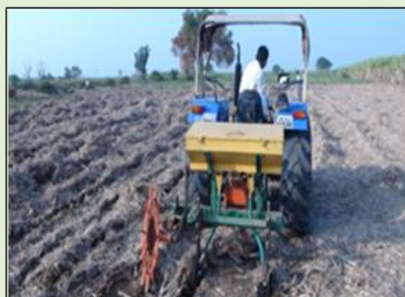
Prototype III: Multifunctional Ratoon Manager Drill (MRMD)
