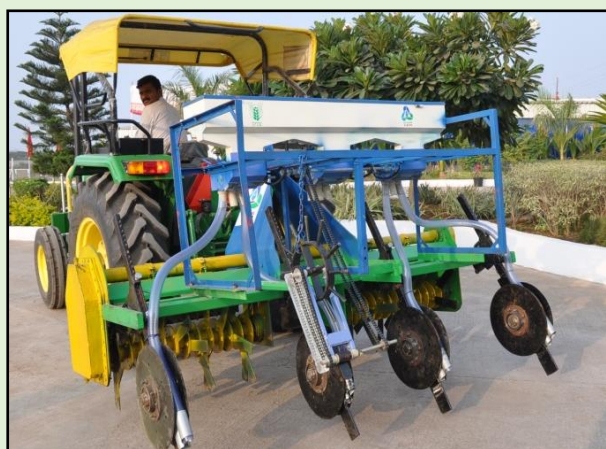
Prototype I: Trash chopper, offbar, root pruner cum fertilizer/ seed drill (ICAR-NIASM)
