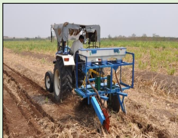
Prototype II: SORF machine- a upgraded version of ratoon management device
