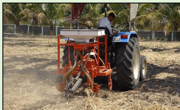
Band placement of fertilizers and sowing of intercrop with SORF machine
