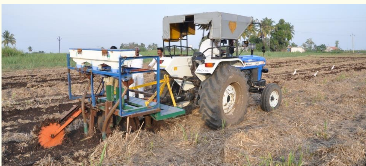
Prototype-II: SORF(Stubble shaving, off baring, root pruning and fertilizer placement)
