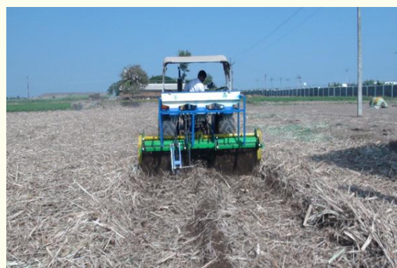
Prototype-I: Trash chopper–offbar–root pruner–fertilizer drill (ICAR–NIASM)
