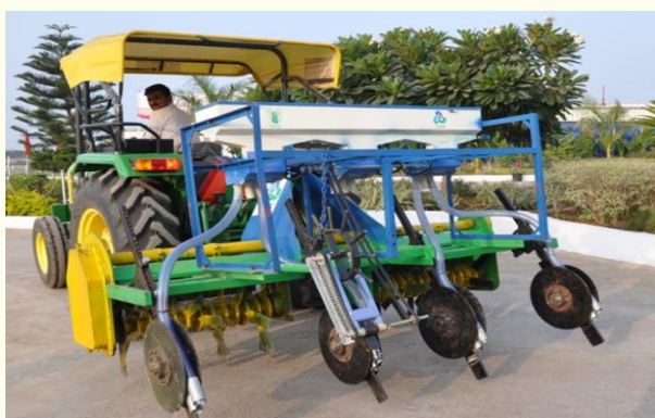
Prototype-I: Trash chopper–offbar–root pruner–fertilizer drill (ICAR–NIASM)
