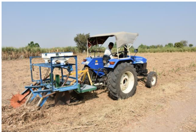
Fig 2. Ratoon management by SORF machine
