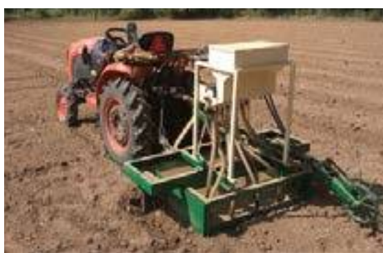
Figure 6.11 : Low HP tractor operated onion seed BBF planter
