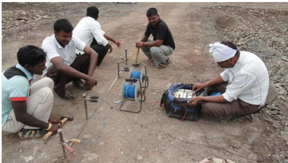
Fig. 6.1. Geophysical Surveys for groundwater exploration using Electrical Resistivity Method at NIASM Site
