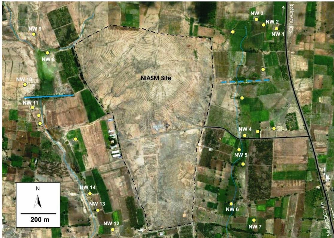
**Fig. 2.2:** Location map of the NIASM site, Malegoan Khurd. Also shown are the locations of the water abstractions structures in the study area. Sample numbers indicated are those used for water quality studies
